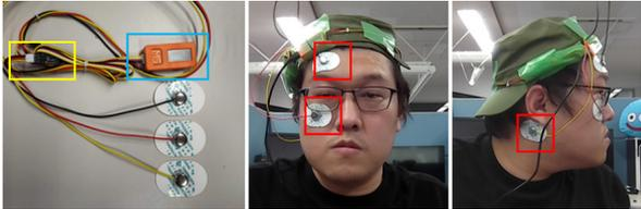
Fig. 1. EOG device (yellow - BioAmp, blue - M5stick-C and red - electrode)
