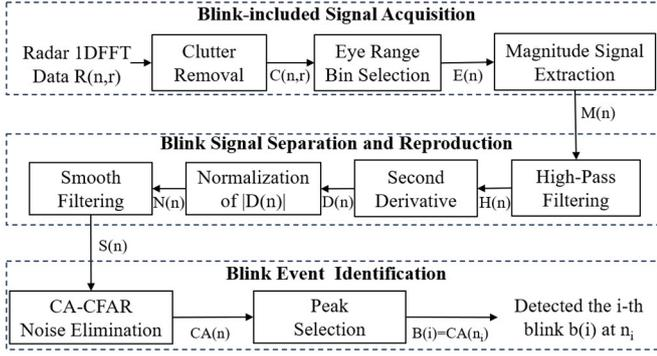
Fig. 5. FMCW radar based blink detection pipeline
