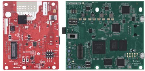
Fig. 10. IWR1843BOOST (left) and DCA1000EVM (right)
