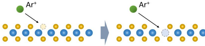
Fig. 2.7 Schematic of Ar-ion beam irradiation before and after S vacancy introduction.
