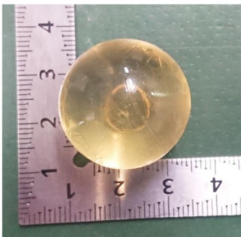
Fig. 3-17 Photograph of sphere gelatin projectile.
