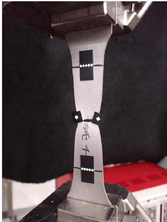
Fig. 3-12 Photograph after tensile test.
