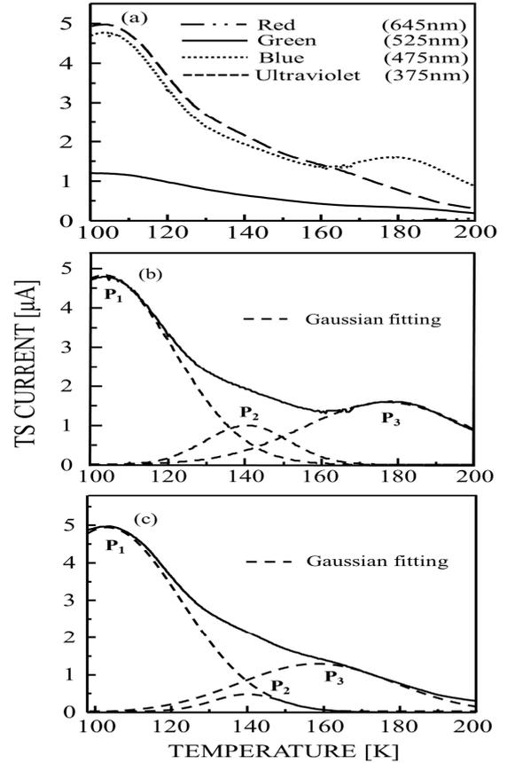
**FIG. 2** TSC spectra (a) taken using LEDs with various wavelengths. Spectra (b) and (c) were measured using blue and ultraviolet LEDs.
