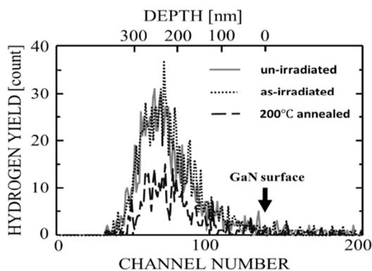
**FIG. 1** Hydrogen in un-irradiated, as-irradiated and  $200^\circ\text{C}$  annealed GaN evaluated by ERDA.
