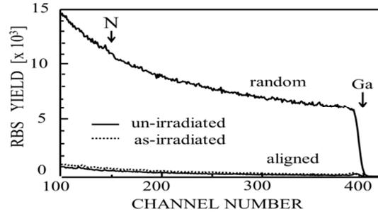
**FIG. 3** Aligned and random RBS spectra for un-irradiated and as-irradiated GaN using 1.5 MeV  $\text{He}^+$  ions.
