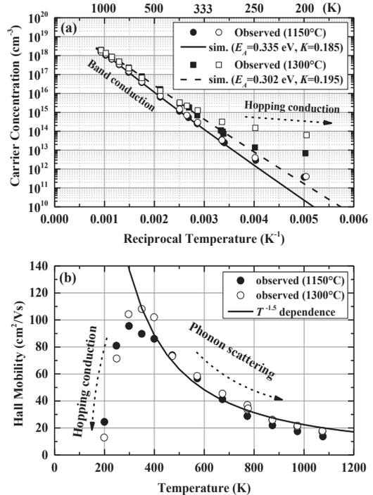
Fig. 2: Experimental and best-fitted carrier concentrations (a), and Hall mobility (b) for the B-implanted sample at RT followed by subsequent annealing at 1150 and 1300°C.
