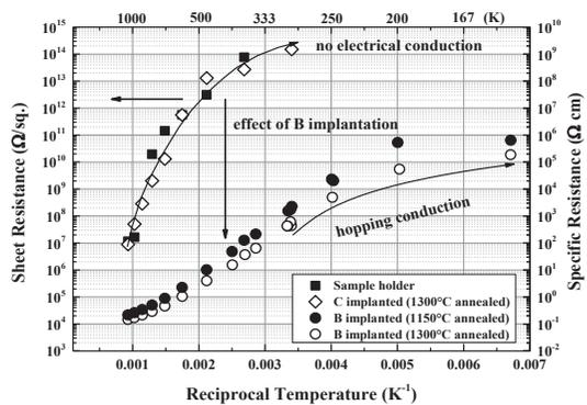
Fig. 1: Sheet and specific resistance for the B-implanted samples at RT followed by 1150 and 1300°C annealing. For reference, the sheet resistances of the sample holder and C-implanted sample after 1300°C annealing are shown.
