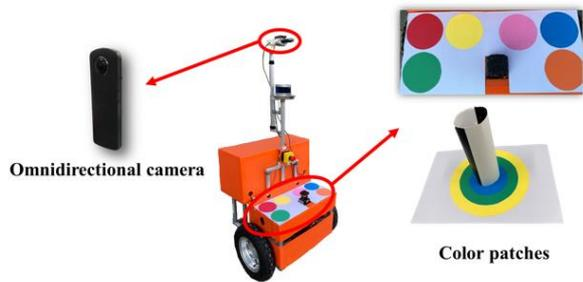
Fig.9 The robot and sensor and color patches used for research
