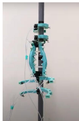
Fig.2 TAOYAKA-SII: a Pipe Climbing Robot with a Soft Body
