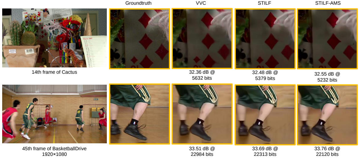
Figure 4.16: Qualitative comparison of VVC [2], STILF [1], and STILF-AMS (ours) at QP of 37. Cactus POC 14 and BasketballDrive POC 45 coded under LDP configuration.
