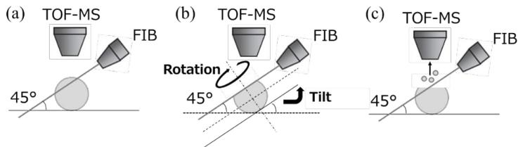
Figure 2: Eucentric rotation system in this study
