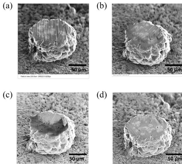
Figure 5: Processed cross section from the first to the fourth direction. (a) shows the machined cross section in the first direction (rotation  $0^\circ$ ), (b) in the second direction (rotation  $45^\circ$ ), (c) in the third direction (rotation  $30^\circ$ ), and (d) in the fourth direction (rotation  $-30^\circ$ ).
