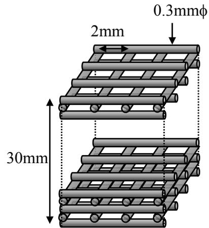
Fig. 4. Collimator-B
