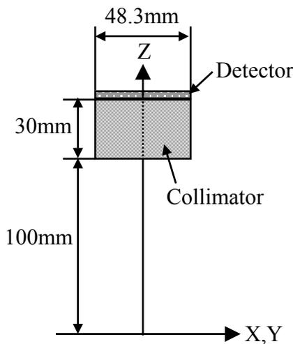
Fig. 2. Simulation geometry
