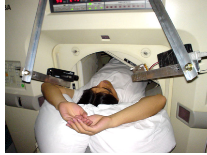
Fig. 10. Gamma camera system and FGD sensor (right) with the ITV camera (left)
