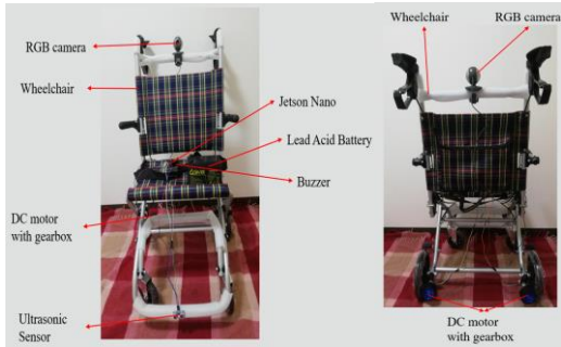
Fig. 3.a. Front view and 3.b. Back view of the constructed prototype.
