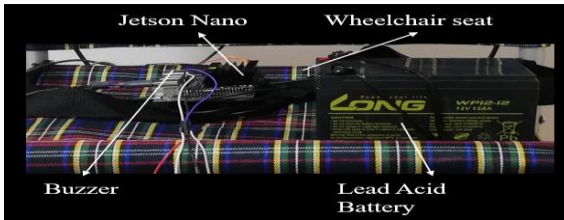
Fig. 3.c. remaining hardware of the constructed prototype.
