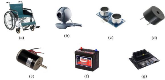
Fig.1 (a) Wheelchair. (b) RGB camera. (c) Ultrasonic sensor. (d) Buzzer. (e) DC motor. (f) Rechargeable battery. (g) NVIDIA Jetson Nano.
