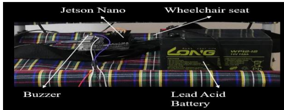
Fig. 3.c. remaining hardware of the constructed prototype.
