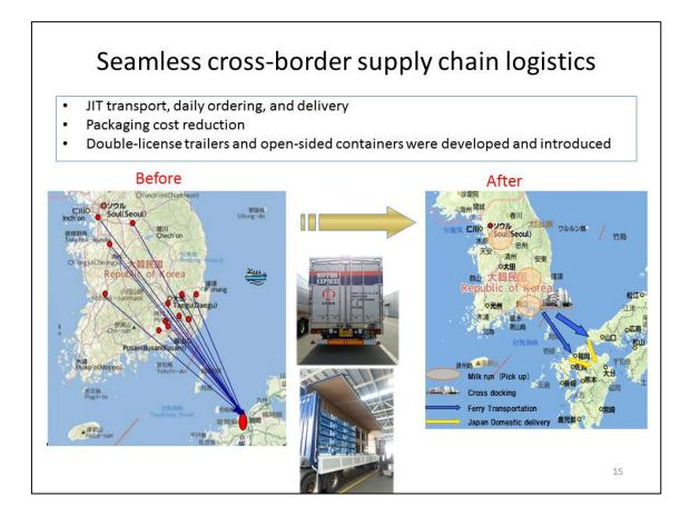
In the past, transportation was managed by each parts supplier, and it took a long time for every shipment to arrive. Now, parts are collected daily via a 'milk run,' gathered at the cross-docking center in the Busan FTZ, and then loaded onto a roll-on/roll-off (RORO) ferry operating between Busan and Kyushu.
