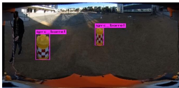
Fig.16 Results of obstacle detection by using YOLOv3-tiny
