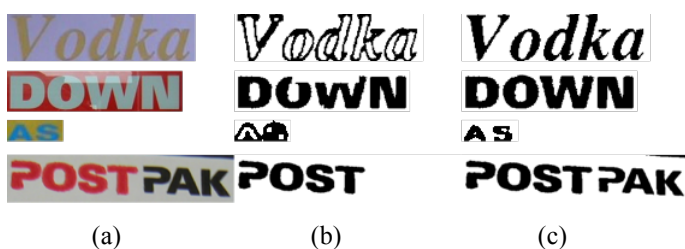
Fig. 12. Examples of mistakenly binarized images due to the second cause. (a) Original color images. (b) Selected binarized images. (c) Optimally binarized images.
