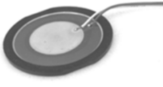
Fig. 1. Piezo device used in a buzzer.
