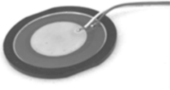
Fig. 1. Piezo device used in a buzzer.
