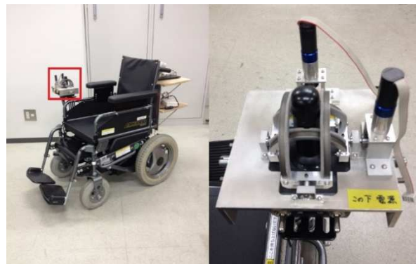
Fig.7 Electric wheelchair and joystick control device
