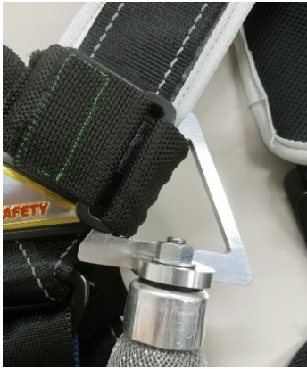
Fig.15 Triangular attachment implement
