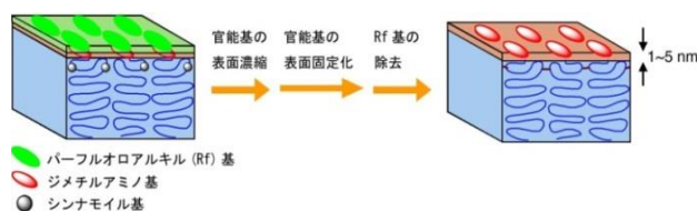
Fig.1. Preparation of film surface concentrated with tert -amino groups
