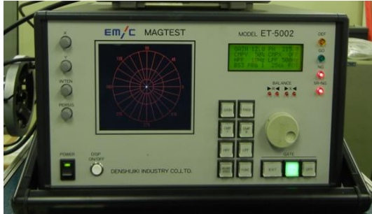
Fig.4. ET-5002 ECT signal processor made by Emic (Denshijiki Industry Co., Ltd).
