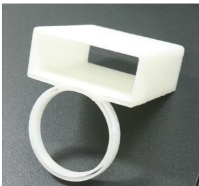
Fig.5 Method of mounting the sensor
