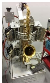
Fig.1 External view of the automatic saxophone robot
