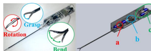
Fig. 3 Forceps manipulator for SPS
