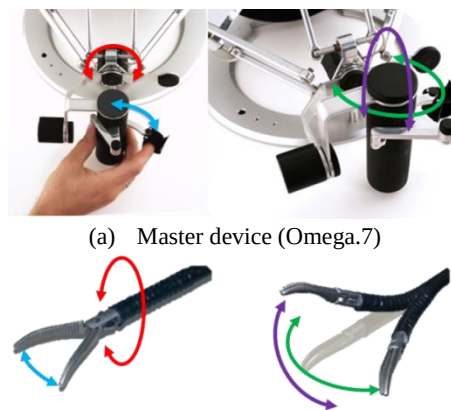
Fig. 4 Manipulations of Omega.7 and forceps manipulator
