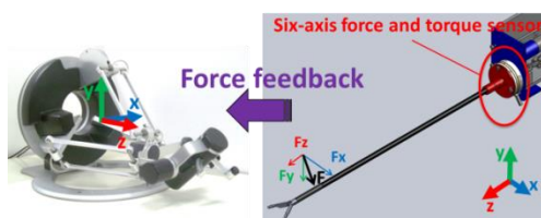
Fig. 5 Force sensing and its realization in Omega.7
