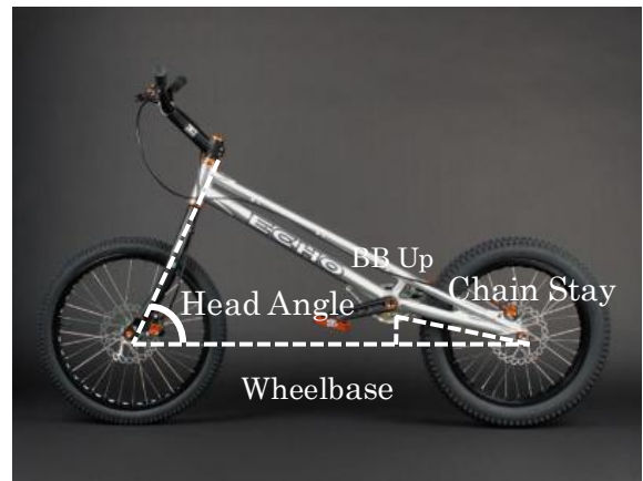
Fig.5-1 Define of each part of a bicycle
