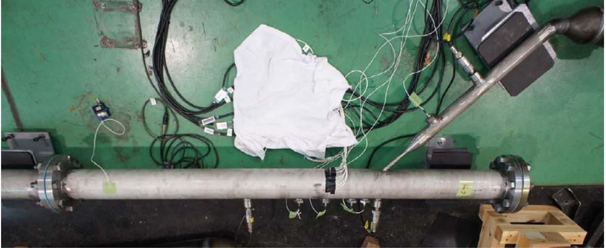
Fig.4.9 Experimental piping system (4 inch x 0.25 inch with 45 degree combining angle tee)
