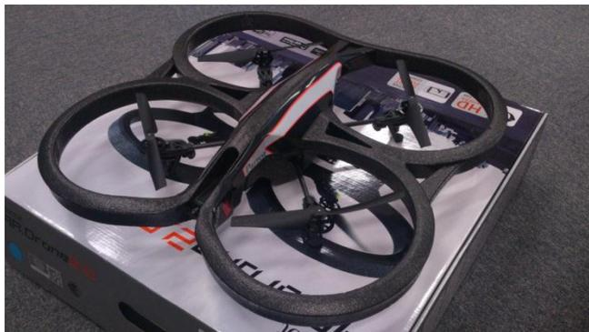
Fig.8 Flying robot, AR.Drone2.0(Parrot.inc)
