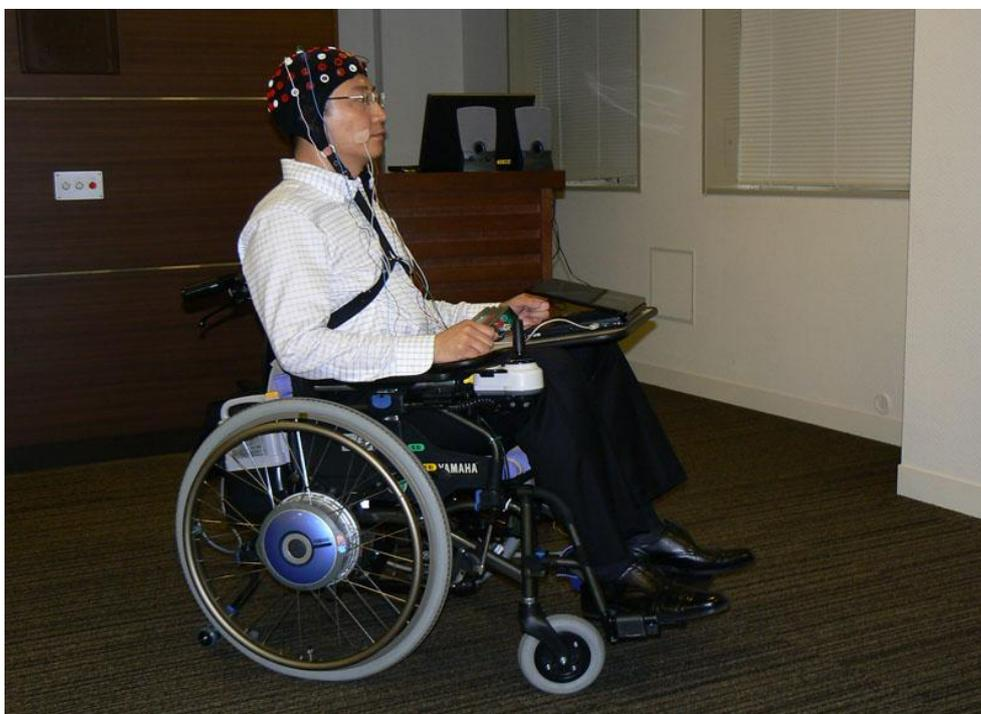
Fig.3-1 Control of the Wheelchair by EEG Signals [7]
