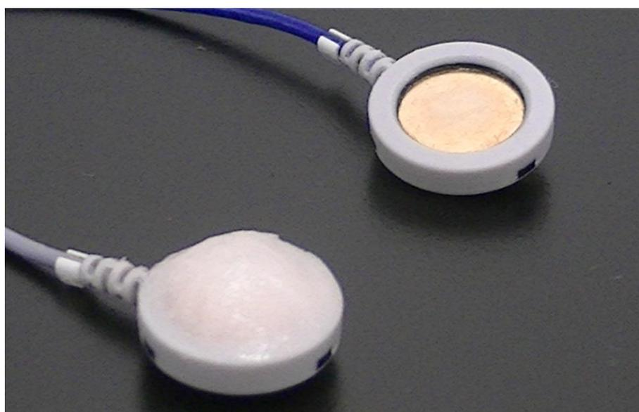
Fig.2-3 Active electrodes
