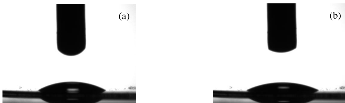
Fig.3-5-6. Contact angle of n -dodecane droplets on P(St-FI)- b -PFMA-2 film after soaked in n -dodecane (2 cycle) (a) P(St-FI)- b -PFMA-2 film [1sec], (b) P(St-FI)- b -PFMA-1 film [120 sec].
