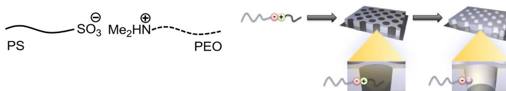
**Figure 1-2.** Representation of the strategy used to prepare nanoporous thin films from blends of mutually interacting end-functionalized homopolymers.
