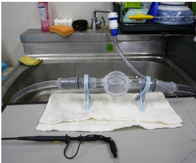
Fig. 32 Experiment using piezoelectricity ceramics flowmeter
