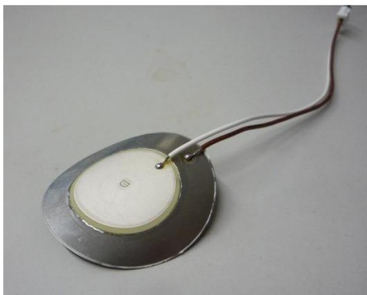
Fig. 10 Piezoelectricity ceramics
