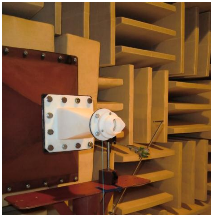
Fig.3.18 Installation of tested nozzle
