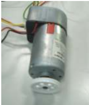
Fig.14 Motor with a pulley
