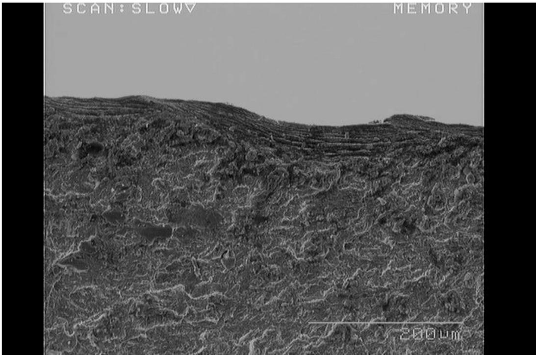
(f)A側 左側段差の疲労き裂発生位置
