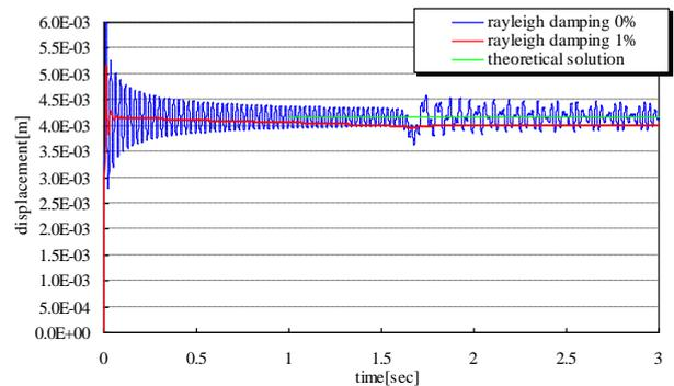
Fig.11 Displacement behavior of nod 1 (1D comparison)
