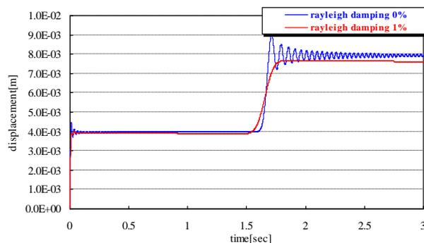
Fig.6 Displacement behavior of nod 100 (1D with CIP)
