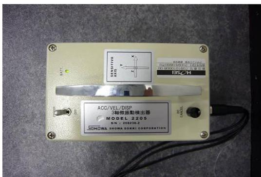
Fig.3 Three axis vibrograph
