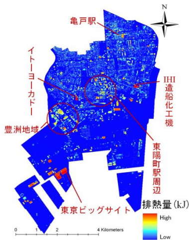
Fig 3.1. Building Heat Release Distribution Map
