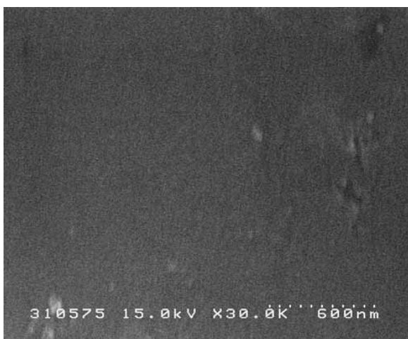
Fig.13 SEM images of MBG surfaces before immersion in SBF.
