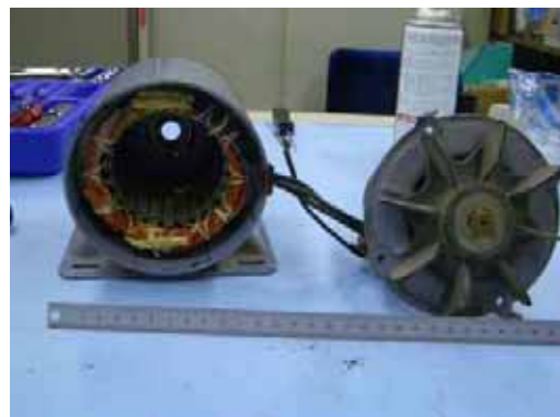
Picture2. Breakup of the generator 1
