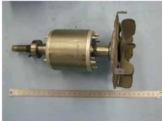
Picture3. Breakup of the generator2
