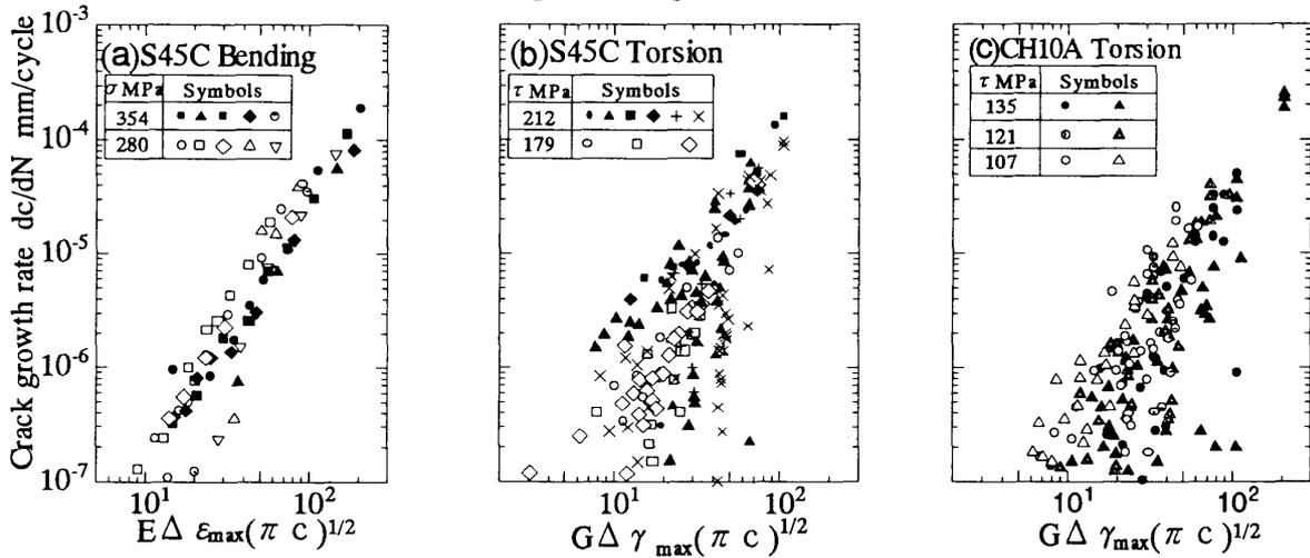
Fig.4 Crack growth rate vs.  $E\Delta\epsilon_{max}(\pi c)^{1/2}$  or  $G\Delta\gamma_{max}(\pi c)^{1/2}$ .
