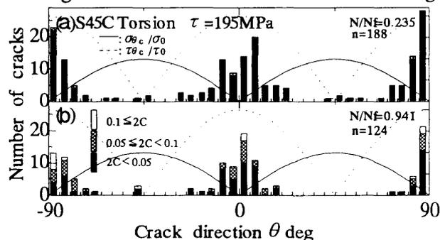
Fig. 2 Distribution of microcracks under torsion.
