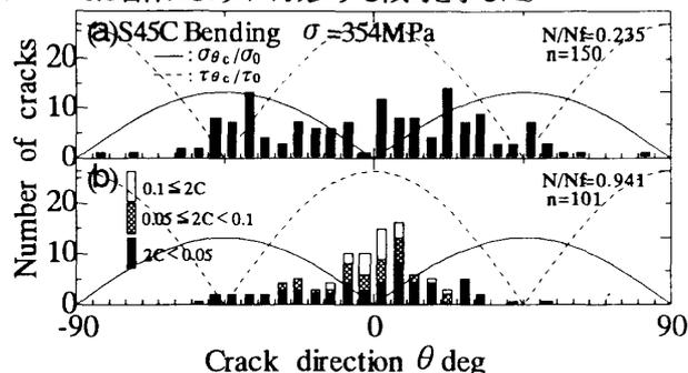
Fig. 1 Distribution of microcracks under bending.
