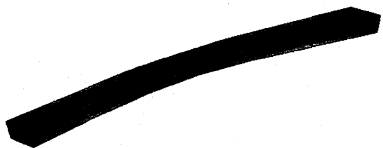
Fig. 3 Experimental Mode Shape No. 1 (Double end free support)
