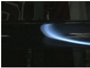
Equivalence ratio of combustion tube \phi = 0.65 Equivalence ratio of injection mixture \phi = 0.55
