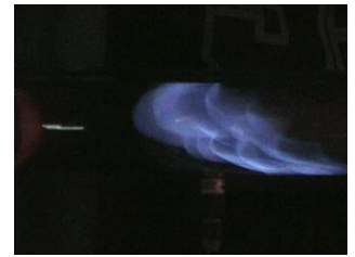
Equivalence ratio of combustion tube \phi = 0.65 Equivalence ratio of injection mixture \phi = 0.50
