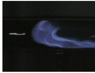
Equivalence ratio of combustion tube \phi = 0.60 Equivalence ratio of injection mixture \phi = 0.55
