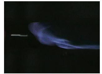
Equivalence ratio of combustion tube \phi = 0.55 Equivalence ratio of injection mixture \phi = 0.60
