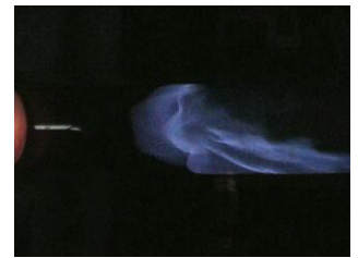
Equivalence ratio of combustion tube \phi = 0.60 Equivalence ratio of injection mixture \phi = 0.60
