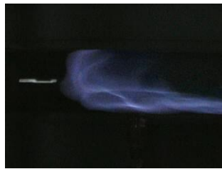
Equivalence ratio of combustion tube \phi = 0.60 Equivalence ratio of injection mixture \phi = 0.65
