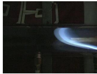
Equivalence ratio of combustion tube \phi = 0.65 Equivalence ratio of injection mixture \phi = 0.50
