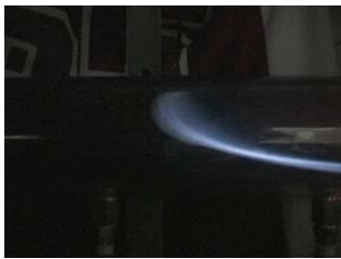
Equivalence ratio of combustion tube \phi = 0.55 Equivalence ratio of injection mixture \phi = 0.55
