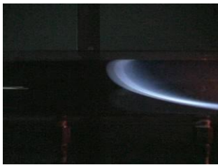
Equivalence ratio of combustion tube \phi = 0.60 Equivalence ratio of injection mixture \phi = 0.65
