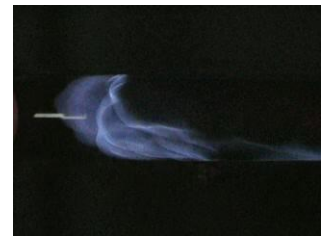
Equivalence ratio of combustion tube \phi = 0.55 Equivalence ratio of injection mixture \phi = 0.50
