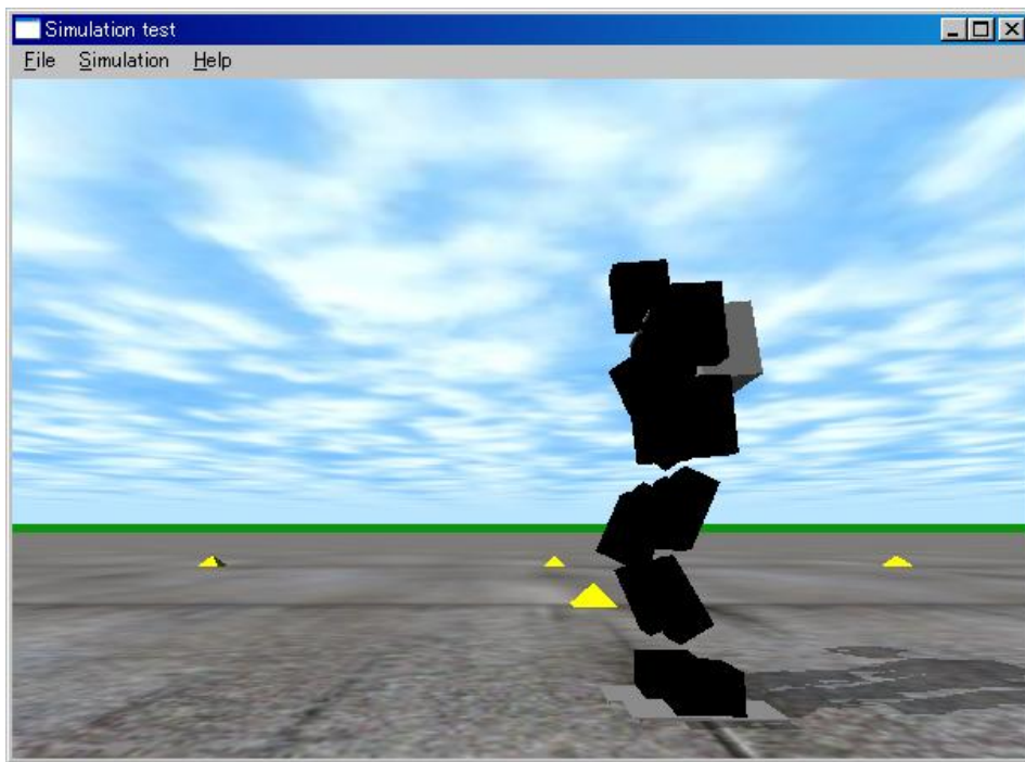
Fig. 9 Simulation screen of walking control by using ODE
