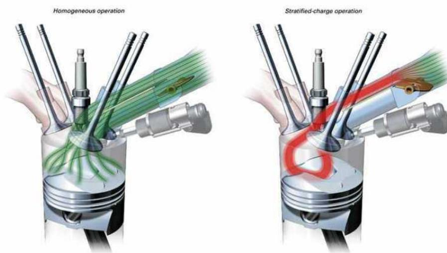
**Fig. 14 Homogeneous combustion and Stratified charge combustion**
