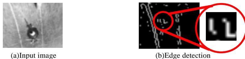
Fig.36 The case that lawn was detected as pothole by using Hough transform
