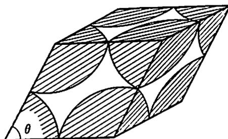
Fig. 2 Slichter's unit cell
