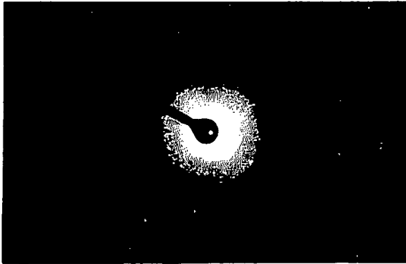
Fig. 3 An electron diffraction pattern of amorphous selenium film prepared by vacuum evaporation.
