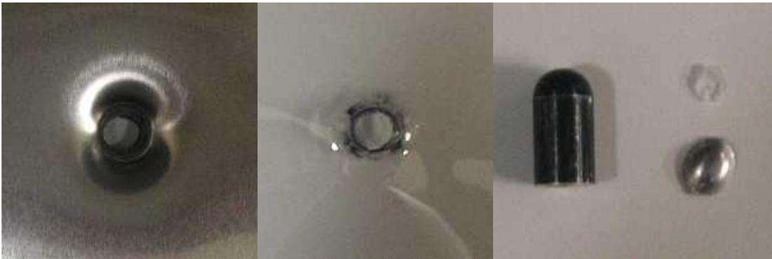
Fig.6-6 Back view of target(Al+PC).
