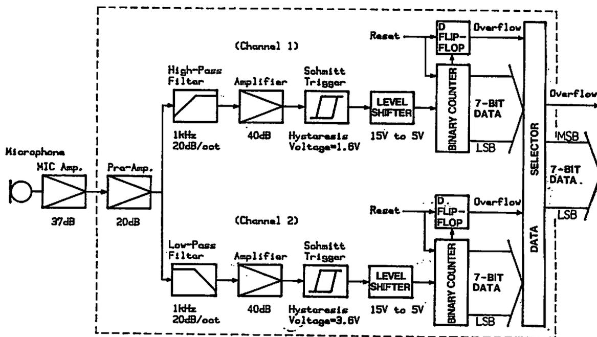
Fig. 3 Block diagram of the preprocessing hardware.
