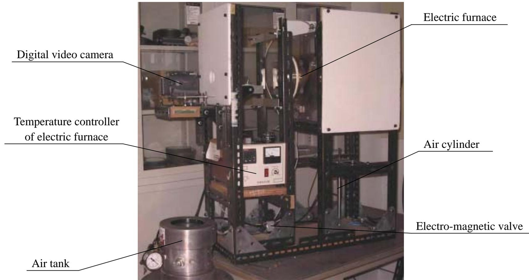
Fig . 2-2 Experimental assembly
