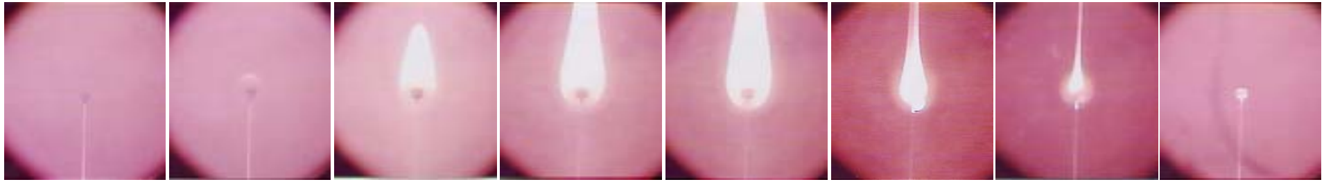
Fig.4 Direct photographs on behavior of fuel sphere at 750°C of ambient temperature and 15% oxygen concentration(vol)
